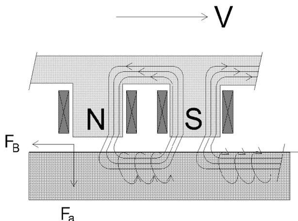
**Figure 1 Braking ( $F_B$ ) and attractive ( $F_a$ ) forces**
