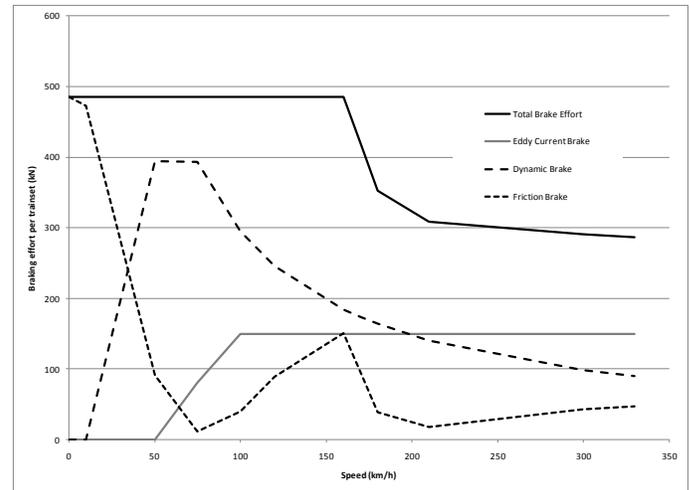
Figure 5 Representative brake blending curve
