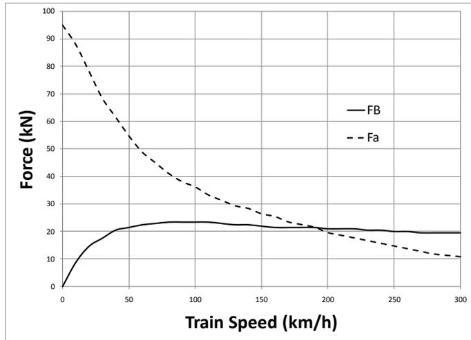
Figure 3 ECB truckset forces with EB energization
