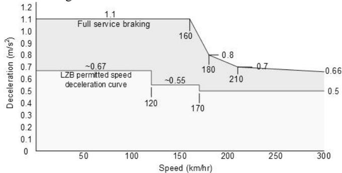
Figure 4 ICE 3 braking rates [7]
